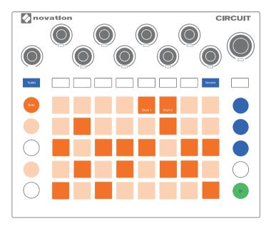
Press pads to turn steps on and off for Drum 1 and 2. You will hear the effect as the play position passes over the step.
