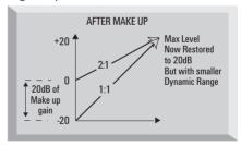
dynamic range of the input and in so doing makes the signal quieter. Using the Make up control restores the volume of the compressed signal.
