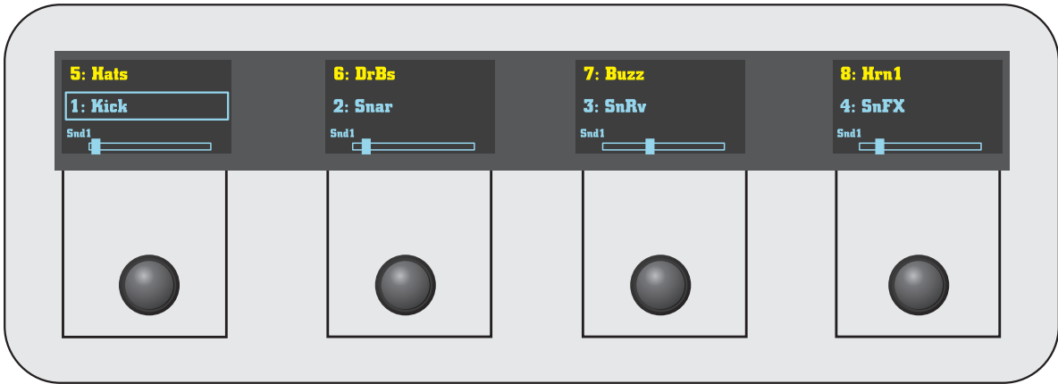
AUX mode (channels 1 to 4) - controlling Send 1:
