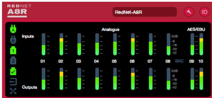
The illustration above shows a RedNet A8R with signals present on all input and output channels. The unit has a single PSU input, single network input and a locked network connection.
