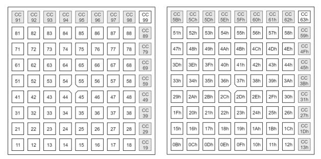
The top row's Session and Custom buttons are not available for control by the DAW, however they still send the corresponding CC messages on interaction, allowing the DAW to catch relevant events as the user interacts with the device (layout changes). All the other pads and buttons (as well as the logo) are available, and reflect the state set up by the corresponding MIDI events.
