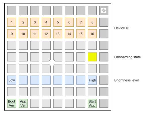
The top two rows of pads can be used to set the USB device ID of the Launchpad Mini [MK3]. The device ID ranges from 1 to 16, the selected ID is represented by a brightly lit pad. The default ID from factory is 1. If more than one Launchpad Mini [MK3] is used on the same USB, each should have a different device ID selected.
