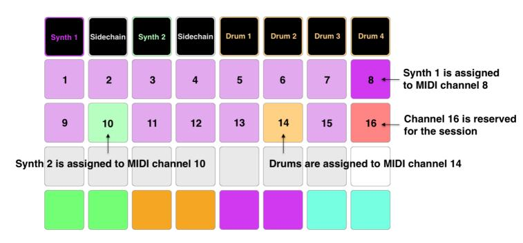
The placement of the purple, green, and orange pads in the top two rows show the MIDI channel each track is currently assigned to.
