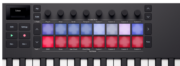
The Launchkey Mini 37 pads reflecting the track select and record arm states on the pads.
