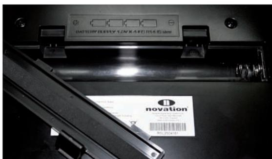
Battery Compartment: Found on the bottom of the unit, this compartment holds four 1.5V IEC R14 (C size) batteries for powering the ReMOTE ZeRO SL.
