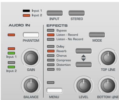
There are two completely independent multi effects processors available, one for Input Channel 1 and one for Input channel 2. An example is presented using a Microphone plugged into Channel 1 and a Guitar plugged into Channel 2.
