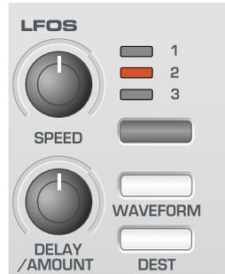
There are two LFOs - Low Frequency Oscillators - available on the KS Synth. These produce regular electronic variations which are too low to be heard when converted into audio vibrations. They can modify various elements of the sound, producing regular changes in pitch (vibrato), pulse width or filter Cut off.
