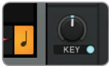
Hold **SHIFT** and press the **TEMPO** encoder to activate key lock.
