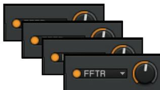
**FX 1 PARAMS, FX 2 PARAMS, FX 3 PARAMS, FX 4 PARAMS:** use to change the function of the 4 knobs above, when none of **FX PARAMS** LEDs are on then the knobs control the dry/wet balance of units 1 to 4. For example, if the **FX 1 PARAMS** button is pressed it will light up to indicate that the knobs function have changed. **Knobs 1 to 4** will now allow control of the advanced control of FX unit 1 represented by horizontal sliders on Traktor's GUI.
