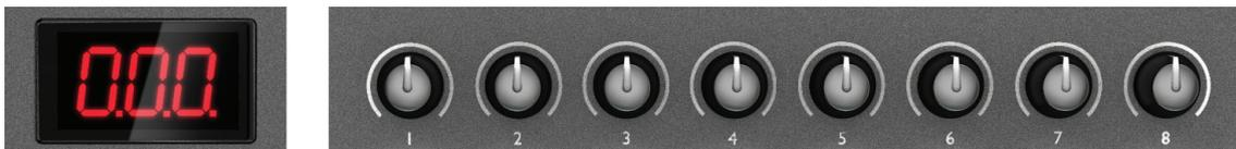
All models have eight rotary controls [6], which like the other Launchkey controllers, may be placed in InControl mode, or used in Basic Mapping Mode. In InControl mode they would typically act as pan controls for a set of eight channels in the DAW's mixer section. In Basic Mapping mode, each rotary control transmits a fixed MIDI CC message. See the MIDI tables on page 24.
