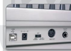
The rear panel provides options to power by batteries or an external power supply, rather than over USB, as well as featuring a MIDI Out for connecting to additional MIDI equipment
