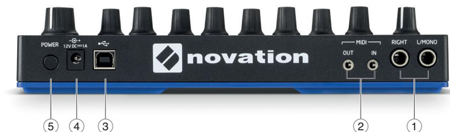
① **L/MONO** and **RIGHT** – Circuit’s main audio outputs on two ¼” TS jack sockets. Max. output level is +5.3 dBu (+/-1.5 dBu). With no plug in the **RIGHT** socket, the **L/MONO** socket carries a mono mix of L and R channels. The internal speaker is muted when a plug is inserted into either of the main output sockets.
