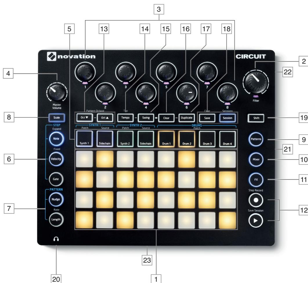
**1** 32-pad playing grid – a 4 x 8 matrix of rubber pads; internally illuminated with RGB LEDs. Depending on the view selected, the grid may be “split” into logical areas with different functions.
