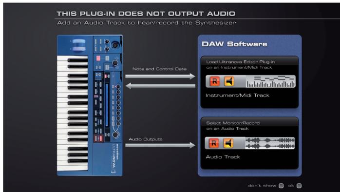
**NOTE:** Although the UltraNova Editor is an Instrument plug-in, it is important to understand that the Editor is not an audio source; it is a means for transferring control data. The source for the audio is the UltraNova, thus to hear/record audio a dedicated audio channel will need to be used in the music software.
