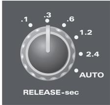
**\* TIP!** Use faster release times if you want to get the compressor out of the way quickly, and produce very obvious compression which can lead to “pumping”. For your drum bus, try starting at **0.1 sec** and then work backwards until you get a suitable balanced effect.
