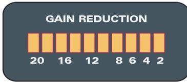
This is a 10-segment LED bargraph meter, indicating the amount of gain reduction applied when compression is active. The scale shows 2dB to 20dB of compression.
