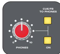
On the front panel, use the **ON** switch (22) to activate the headphone output.
