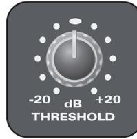
This control sets the threshold level, and is variable from -20 to +20dB.
