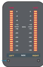
The LEFT and RIGHT MIX meters are actually fed from the monitor output (after the MONITOR SOURCE selector but before **VOLUME**, etc). This is often known as “follow monitor” metering, which allows you to meter any source, not just the main mix.
