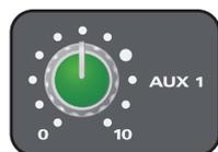
This control sets the level feeding the AUX 1 (or AUX 2) bus. Send levels can be adjusted individually, channel-by-channel.
