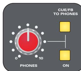
Turn on the **CUE/FB TO PHONES** switch in the monitor section - this routes the cue output to the headphone connector on the rear panel.
