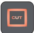
Press this switch to mute the monitor output. This is a global cut that disconnects both the main and alternate loudspeaker outputs.
