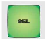
The **SEL** switch selects the fader strip. It is used in conjunction with the SELECT MODEs on the Control Surface Panel to perform a number of functions.
