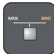
This switch determines whether you are monitoring the main mix or the output of the **MONITOR SOURCE** selector. One of the options must be active:
