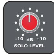
In either **AFL** or **PFL** mode, use this control to trim the level of the solo bus. Level may be trimmed by +/-10dB.
