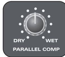
This control “crossfades” between the uncompressed and compressed signal, a technique known as parallel compression:
