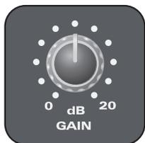
This control adjusts the gain after compression, and is variable from 0 to 20dB. It is very useful for restoring the output level, which will have been reduced by active compression.
