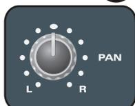
This control pans the source onto the stereo cue bus.
