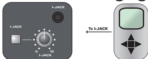
This stereo mini jack input (8) is designed for connecting portable music players. This is a stereo unbalanced input with approximately 10k Ohms input impedance.
