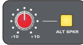
A second set of loudspeakers may be connected to the alternate outputs (ALT SPKR L/R). Applications include nearfield or mini “grot-box” monitors.
