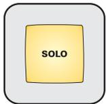
The **SOLO** switch places the channel into one of three solo modes: AFL (after-fade listen), PFL (pre-fade listen) or SIP (solo-in-place). The mode is selected globally from the master section, see page 40
