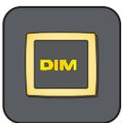
Press this switch to dim the monitor output. The amount of dim is set by the **DIM LEVEL** control (11).
