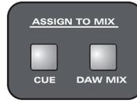
The **ASSIGN TO MIX - CUE** switch, in the master section, routes the cue bus onto the main mix. Note that ALL cue sends feed the main mix when this switch is active.
