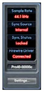
The Device Status section shows information about the sample rate, synchronisation and driver status of the Saffire PRO 40. The desired sample rate can be set as well as external synchronisation options for using the Saffire PRO 40 with external digital devices.
