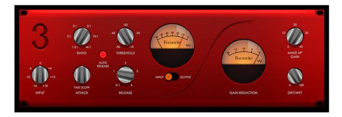
A compressor essentially acts like an automatic volume control, turning down the volume of a signal if it gets too loud. This reduces variation between loud and quiet passages, as it automatically reduces the gain when the signal exceeds a given volume, defined as the threshold. The overall level can then be turned up to make the signal as loud as possible.
