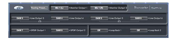
The routing section allows you to set up how the various audio sources in the mixer are to be routed to the outputs.
