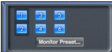
The monitor control enable buttons indicate which outputs are controlled by the monitor section on the GUI directly below the six buttons. The Saffire PRO 24 DSP has two levels of monitor volume control. The software monitor knob can be used to control the level of up to 6 outputs simultaneously. However the physical monitor knob controls the level of outputs 1 and 2 (post software control).
