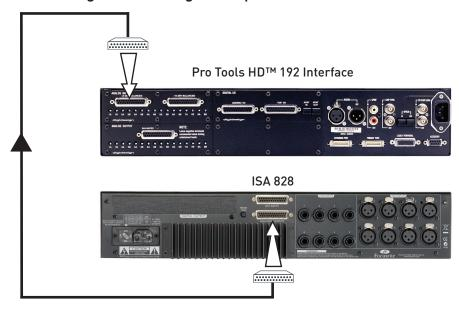
■ Recording from AES Outputs 1-8 to Pro Tools™ HD at 44.1-96kHz
