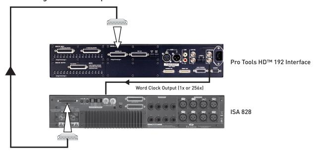
■ Recording from AES Outputs 1-8 to Pro Tools™ HD at 192kHz
