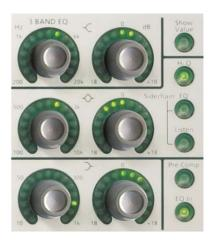
The Liquid Channel™ features a new digital ('modelled' rather than 'convolved') EQ, loosely based on the classic Focusrite sound of the original ISA 110. This is designed to allow small amounts of corrective shaping. All of the EQ settings can be saved, along with those of the mic-pre and compressor, in one of the Program slots (see the DATA SELECT section below).
