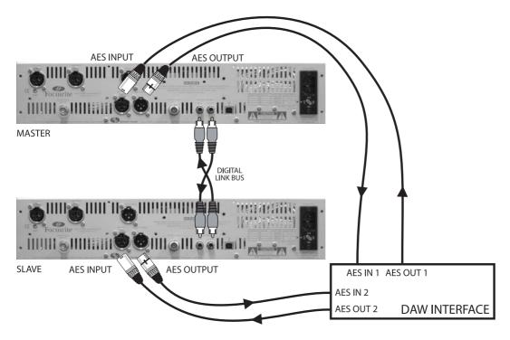
(For 176.4 kHz/192 kHz operation set DAW to send/receive in 'dual wire' mode. See 'Linking Multiple Units' on page 10 for more information.)
