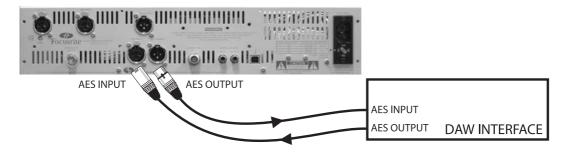
(For 176.4 kHz/192 kHz operation set DAW to send/receive in 'dual wire' mode.)
