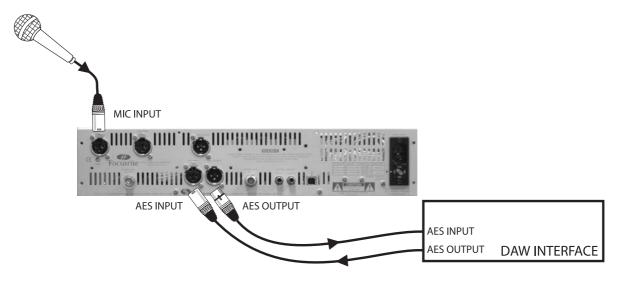
(Liquid Channel™ receives clock from AES connection.)
