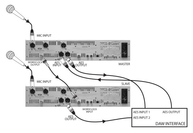
(For 176.4 kHz/192 kHz operation set DAW to send/receive in 'dual wire' mode. See 'Linking Multiple Units' on page 10 for more information.)
