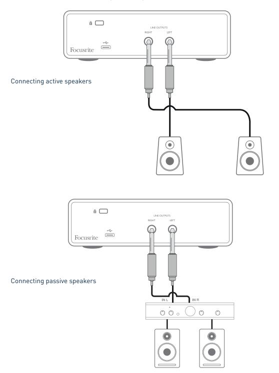
The line outputs are 3-pole (TRS) ¼" (6.35 mm) jack sockets, and are electronically balanced. Typical consumer (Hi-Fi) amplifiers and small powered monitors will have unbalanced inputs, either on phono (RCA) sockets, or via a 3.5 mm 3-pole jack plug intended for direct connection to a computer. In either case, use a suitable connecting cable with jack plugs at one end.
