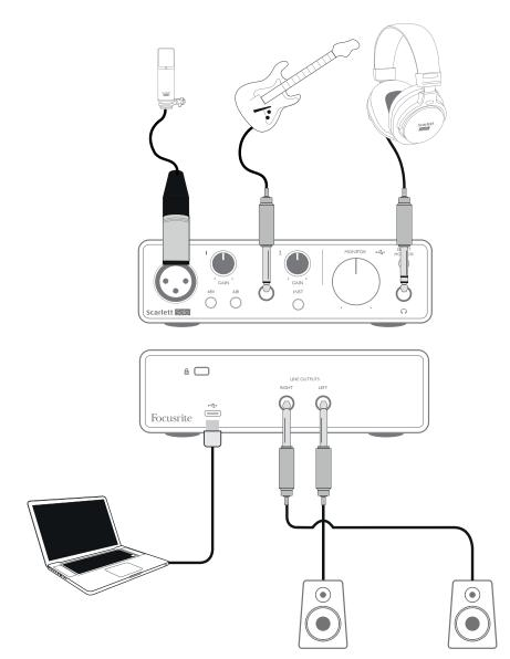
This setup illustrates a typical configuration for recording using DAW software on your Mac or PC. In this case, you would record vocals through Input 1 and guitar through Input 2 into your recording application, while monitoring the playback via headphones.
