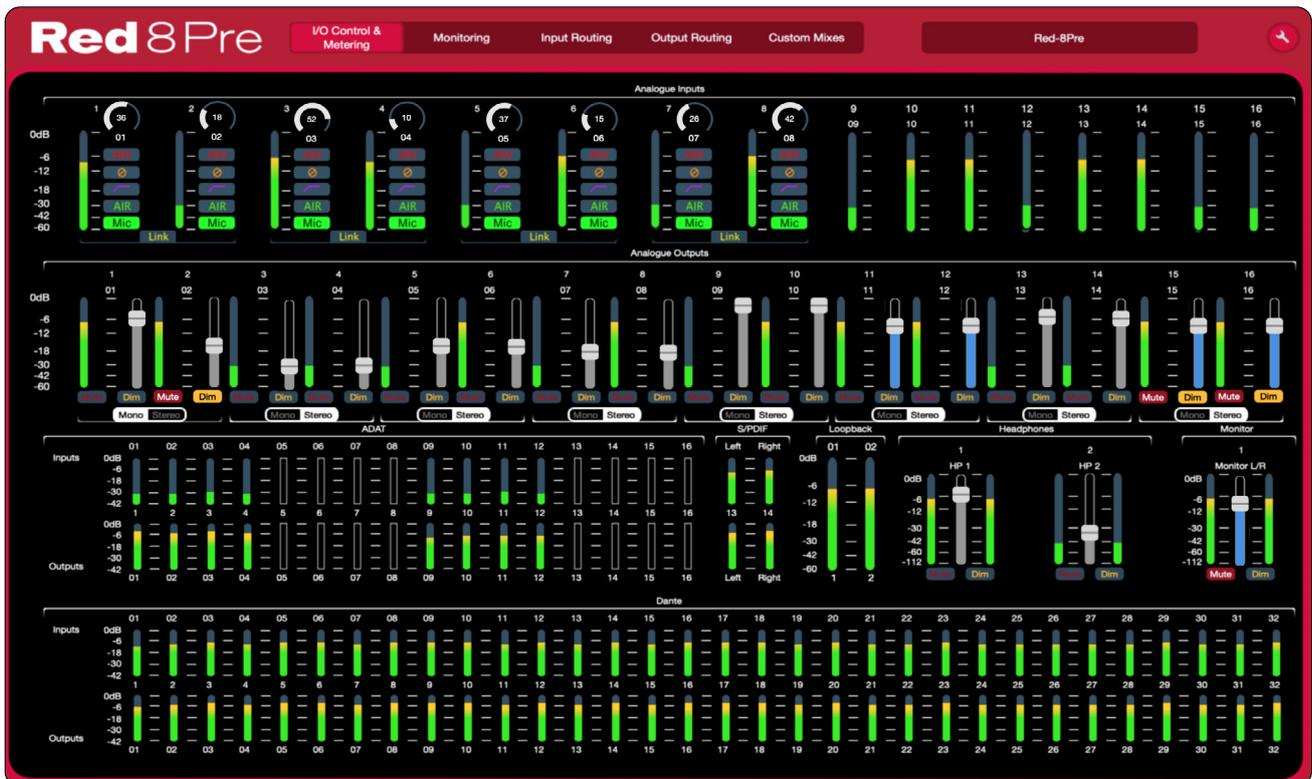
**Analogue Input** – Channel controls operate in the same manner as RedNet devices – See page 9 for details. For channels with gain controls and input functions, the level meter indicates the post-processing signal.
