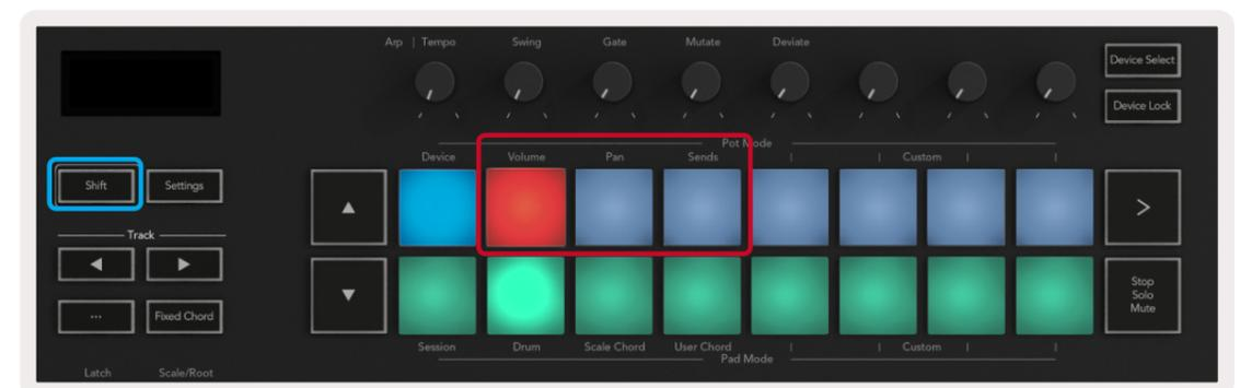
**2.3.1.1 Volume** - This mode allows you to control Track Volumes using the pots. To select this mode, hold the Shift button and press the Volume pad.
