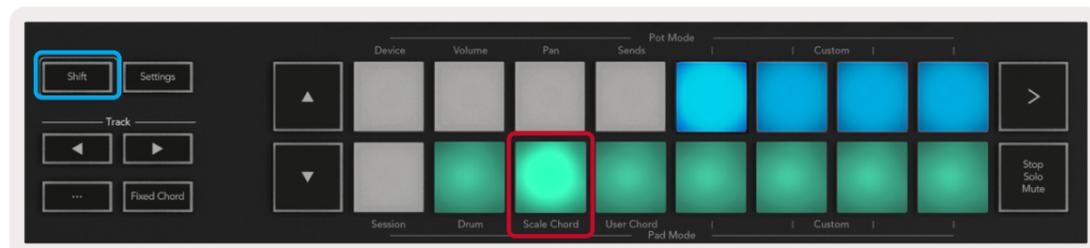
The first and last pad of each row light up more brightly than the middle pads to indicate root chord position. To navigate between pages of chords use the ▲▼ navigation buttons. On the first page the top row of pads are lit blue and contain triads, the bottom row of pads contains 7ths and is lit a darker blue. Pressing the ▼ button will reveal a row of 9ths, with the pads lit up in purple, below this are 6/9ths and the pads will light up in pink.
