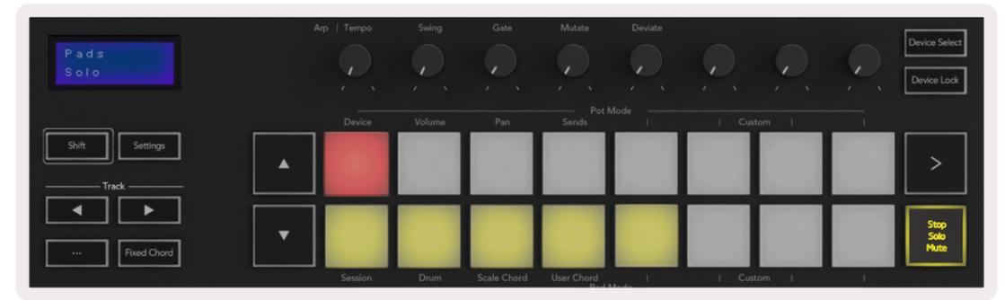
Pressing a red pad will arm that track for recording and it will glow a brighter red. When a track is muted the corresponding pad will become brighter.
