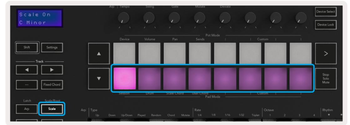
The bottom row of pads will be lit and can be used to select a scale, the selected scale is then shown on the screen. From left to right the pads can be used to select the following scales: Minor, Major, Dorian, Mixolydian, Phrygian, Harmonic Minor, Minor Pentatonic and Major Pentatonic.
