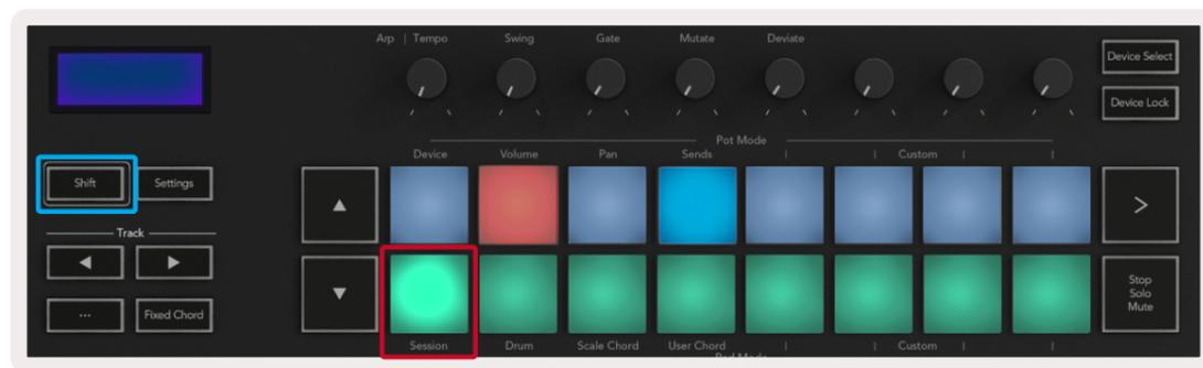
**Record/ Mute mode** - the top row of pads toggles the record arm on the relevant track and will be lit red, the bottom row toggles the track mute and will be lit yellow. The tracks represented by the pads include any sends tracks, the top row of pads will not be lit for sends (buses).
