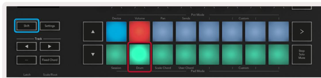
If a Drum Rack is loaded onto the selected Live track, and your Launchkey is in Drum mode, the pads light up the colour of the track. When played the pads will light up green. These pads will play whatever Drum Rack pads are visible on your computer screen. Pressing the ▲▼ buttons scrolls up/ down through a Drum Rack's bank of 128 pads, each press moves up or down the rack in banks of 16.
