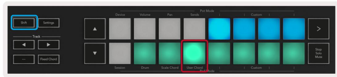
To assign a chord to a pad simply press and hold the pad and press the notes that you want to assign from the keyboard. Up to 6 notes can be assigned to each pad and can be input with individual pushes of the keys, meaning you do not need to hold down all the notes at once so long as the pad is being held.
