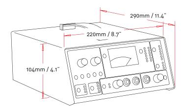
ISA One dimensions are illustrated in the diagram above. Allow for an additional 75mm [3"] behind the unit to allow for cable connections.
