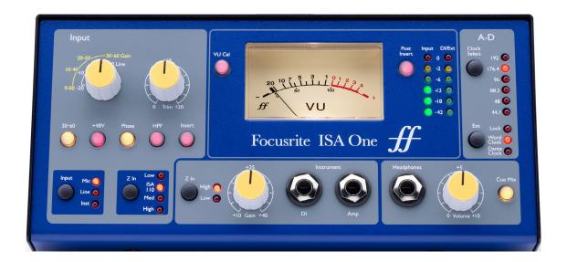
The ISA One is a high quality transformer microphone preamplifier which can be used to record microphone, line-level or instrument sources. Microphone and line-level sources are connected to the rear panel, whilst an independent instrument input can be plugged directly into the front panel jack socket. A local amp or combo can also be connected to the front Amp output jack.
