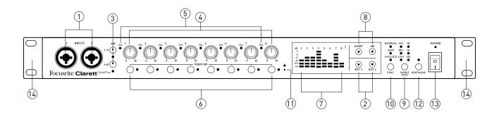
The front panel includes all operational controls, metering for all channels and two input sockets for mic, line or instruments.
