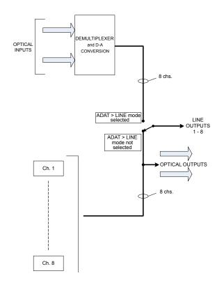
This mode enables the Clarett OctoPre be used to connect an 8-channel ADAT format output (from a DAW, for example) to a set of analogue inputs, typically the channels of an analogue mixing console, to permit such a mixer to be used to mix down DAW tracks.
