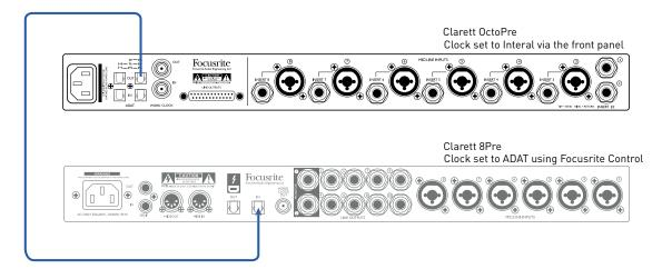
Here the **OPTICAL OUT** on the Clarett OctoPre is connected to **OPTICAL IN** on a Focusrite Clarett 8Pre audio interface with a single optical cable. Both units are running at 44.1 kHz sample rate. The OctoPre's clock source is set to INTERNAL, and the 8Pre is synchronised to it because its clock source is set to ADAT (via Focusrite Control).
