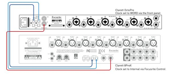
This example shows the same setup as Example 2, but running at a sample rate of 96 kHz ("SMUX-II" mode). Both units must be set to 96kHz; two optical cables are used, carrying four channels of audio each. The Clarett 8PreX is the sync leader as before.
