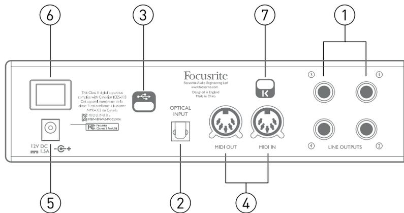
1. **LINE OUTPUTS 1 to 4** – four balanced analogue line outputs on ¼” jack sockets; use TRS jacks for a balanced connection or TS jacks for unbalanced. Line Outputs **1** and **2** will generally be used for driving the main L and R speakers of your monitoring system, while Outputs **3** and **4** can be used for connecting additional line level equipment (e.g., outboard FX processors). The signals routed to all the outputs may be defined in Focusrite Control.
