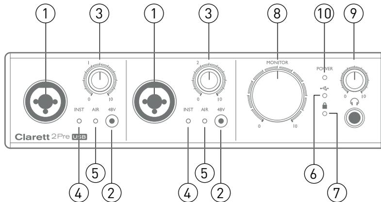
The front panel includes the input gain controls and input connectors for Mic, Line and Instrument signals for both channels, and also the monitoring controls.
