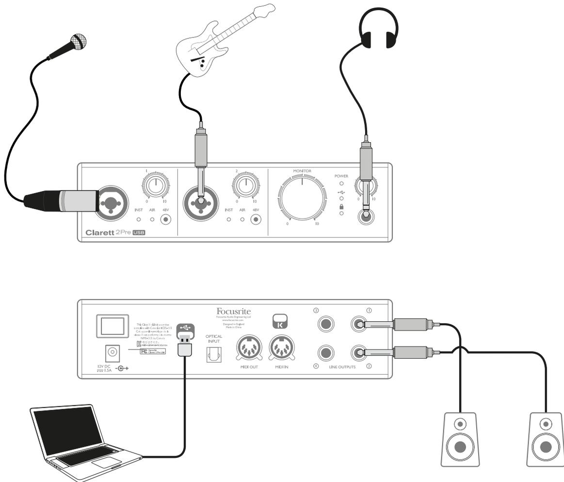
This shows a typical configuration for multitrack recording with DAW software on your computer.
