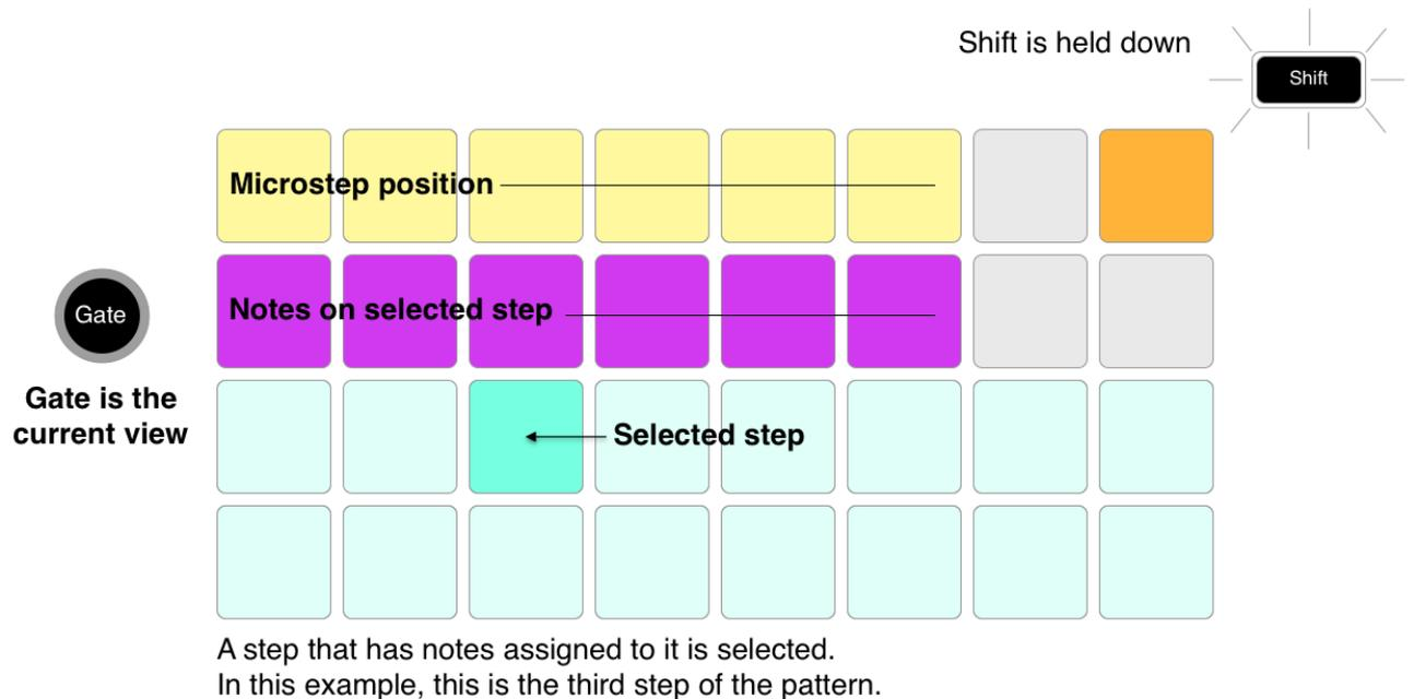
The purple/green pads (Synth 1/Synth 2) represent the notes assigned to the step. Notes are displayed left to right in order of assignment (1<sup>st</sup> note assigned to a step is the leftmost).
