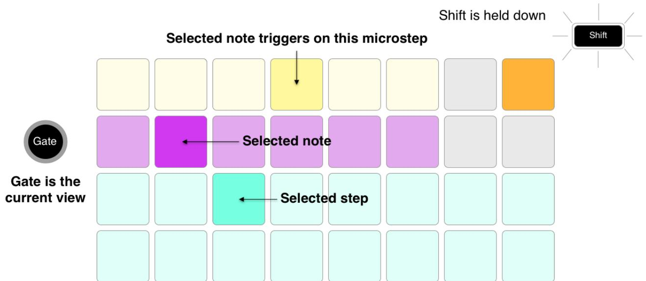
Multiple notes can be selected by simultaneously pressing pads, or by holding down a pad & tapping others. All notes on a step are selected by default before a selection is made.
