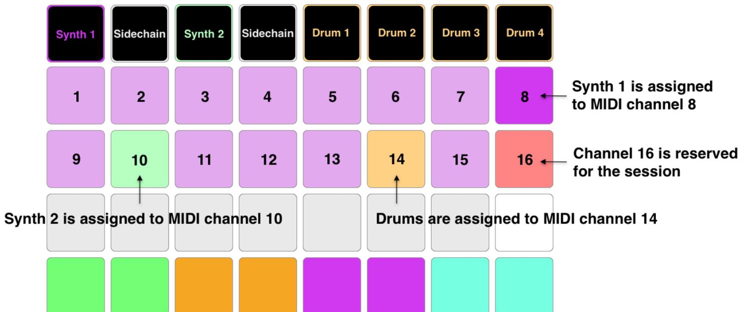
The placement of the purple, green, and orange pads in the top two rows show the MIDI channel each track is currently assigned to.
