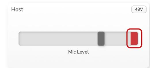
If you see the clip meter appear, turn down the
