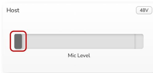
You can click and drag the slider in the software to increase the gain (right) or reduce the gain (left). When you move the
