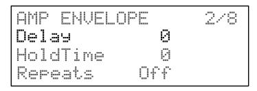
When **Delay** has the default value of 0, the envelopes start their attack phase as soon as Peak receives MIDI. **Delay** inserts a lag between striking the key and the start of the **AHDSR** envelope.
