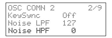
The parameter's default value of zero sets the filter "fully open". The effect of applying this is that each voice will have its own tuning characteristic.
