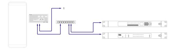
1. Daisy-chained to additional RedNet device in "switched" mode.
