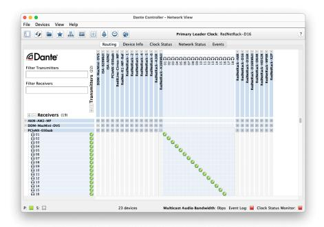
The **Routing** tab is arranged as a cross-point matrix. Audio inputs are listed horizontally (called Dante Transmitters) and audio outputs are listed vertically (called Dante Receivers).
