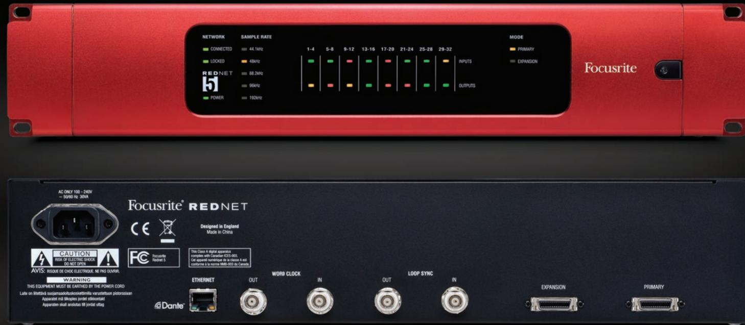
RedNet 5 connects your RedNet system to Pro Tools HD®. Up to six units can be connected to one Pro Tools HDX system, supporting up to 192 channels at 96 kHz or 96 channels at 192 kHz. Three units can be connected to a Pro Tools HD system and two to a Pro Tools HD Native system, delivering 96 and 64 channels respectively at 96 kHz. RedNet 5 is interoperable with other Pro Tools interfaces and no RedNet PCIe card is required.
