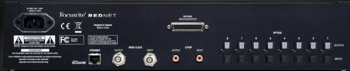
RedNet 3 interfaces your existing digital audio systems and components to the RedNet network, with up to 32 inputs and outputs and full software remote control. The unit includes support for AES/EBU, S/PDIF and ADAT (16 ADAT optical ports support 32 digital channels in and out – even at 96kHz, with S-MUX2) digital audio formats and allows the RedNet system to be synchronised to incoming signal clock or a word clock source.
