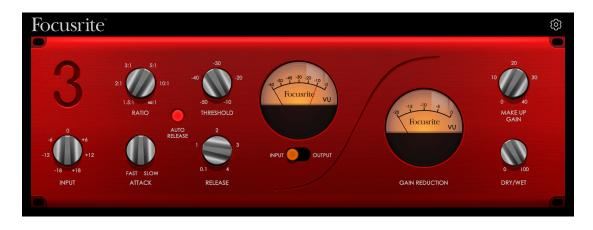
A compressor acts like an automatic volume control, turning down the volume of a signal if it gets too loud. This reduces variation between loud and quiet passages, as it automatically reduces the level when the sound goes above a set volume, the threshold. You can then turn up the overall level to make up the level drop and make the sound louder.
