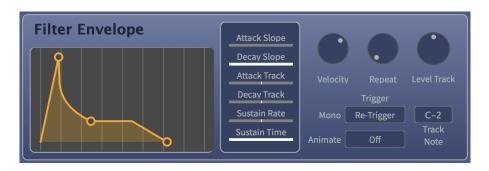
Use the handles on the yellow graph to adjust the ADSR times and levels, and use the faders to the right to adjust the slope of the ADSR.
