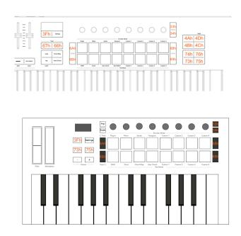
The Control Change indices listed are also used for sending colour to the corresponding LEDs (if the button has any), see Colouring the surface [14].
