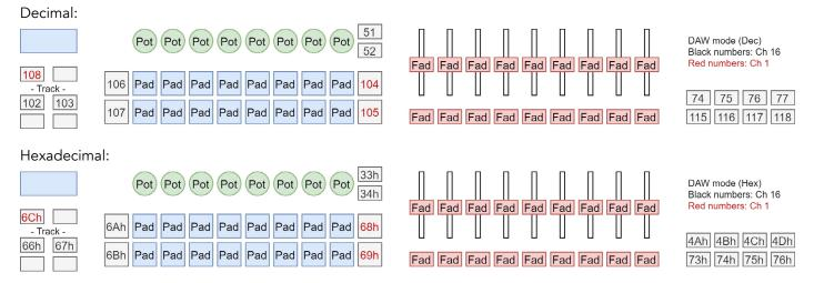
To provide some degree of script compatibility with the Launchkey Mini [MK3], the Scene Up and Scene Down buttons also report back CC 68h (104) and 69h (105) respectively on Channel 16.
