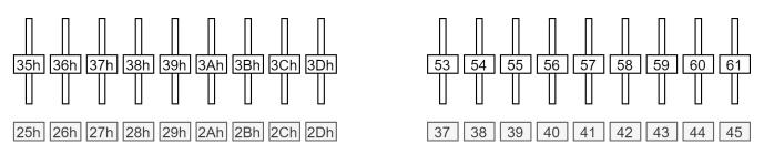
If Continuous Control Touch events are enabled, the Touch On is sent as a Control Change event with Value 127 on Channel 15, while the Touch Off is sent as a Control Change event with Value 0 on Channel 15. For example, the leftmost Fader would send BEh 35h 7Fh for Touch On, and BEh 35h 00h for Touch Off.
