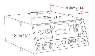
ISA One dimensions are illustrated in the diagram above. Allow for an additional 75mm [3"] behind the unit to allow for cable connections.
