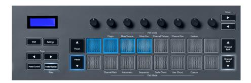
To delete a chord assignment from a pad, hold the **Preset** ▼ button, the pads with assigned chords turn red. Press a red pad to delete the assigned chord, once deleted the pad is no longer lit.
