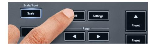
Hold Shift in any pad layout mod while the FL Studio Channel Rack is visible to see the current selection. This applies to Channel Bank Selection, Channel Rack Pot Control and Channel Selection. If you select a Mixer Pot Mode this displays the selected mixer bank.
