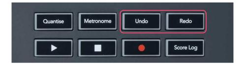
You can press the Undo and Redo buttons on FLkey to trigger FL Studio's undo and redo functions. The FL Studio setting "Alternate undo mode" doesn't affect how these buttons work.
