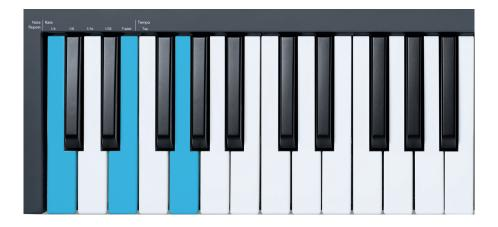
Press and hold the Fixed Chord button press and release C, E, and finally G (a C Major chord). The FLkey stores this as the 'Fixed Chord'. Release the Fixed Chord button.
