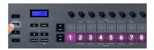
The bottom row of the pads lights so you can select a scale, and the screen shows the selected scale. From left to right, the pads select the following scales:
