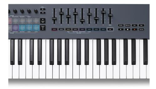
To turn on Solo mode, press the Solo button, the Solo button lights and the fader buttons start dimly lit.
