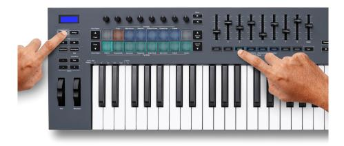
When you move a fader your FLkey 49/61's screen temporarily shows the plugin parameter's name and new value.
