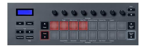
The **Page** ◀ ▶ buttons transpose the chord bank in semitones between -12 and +12, the FLkey's screen displays any changes you make.
