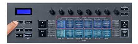
When you enable 'Pickup (takeover mode)' inside FL Studio's MIDI settings, the pot needs to reach the original value before the changes apply to the parameter connected to the current pot.
