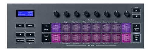
When you press a pad, it lights green and returns to its original colour when released. To change the chord's octave, hold Shift and press the **Page** ◀ ▶ buttons, these provide access to a range of -3 to +3 octaves.
