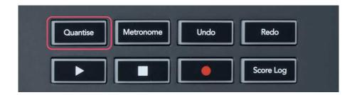
When you press the Quantise button on FLkey it performs the 'quick Quantise start times' function in FL Studio. This quantises all note's start positions in the piano roll for the currently selected Channel Rack channel to the current piano roll snap setting.
