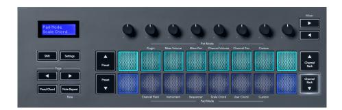
Each row's first and last pad lights up brighter than the middle pads to show the root chord position. To navigate between pages of chords, use the **Page** ◀ ► navigation buttons. This mode has three pages with predefined chords: Triads, 7ths, 9ths, and 6/9ths.
