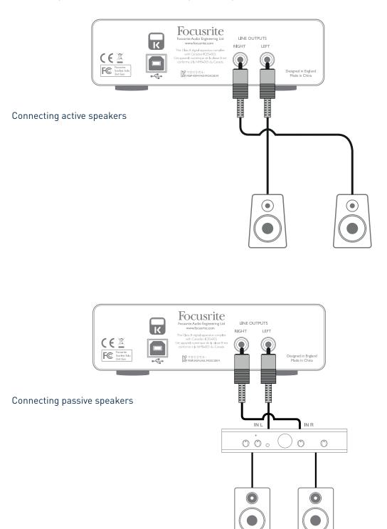
The line output connectors are standard phono (RCA) sockets. Typical consumer (hi-fi) amplifiers and small powered monitors will have inputs on phono (RCA) sockets or a single 3.5 mm 3-pole jack plug (intended for direct connection to a computer). In either case, use a suitable connecting cable with phono plugs (RCA jacks) at one end.
