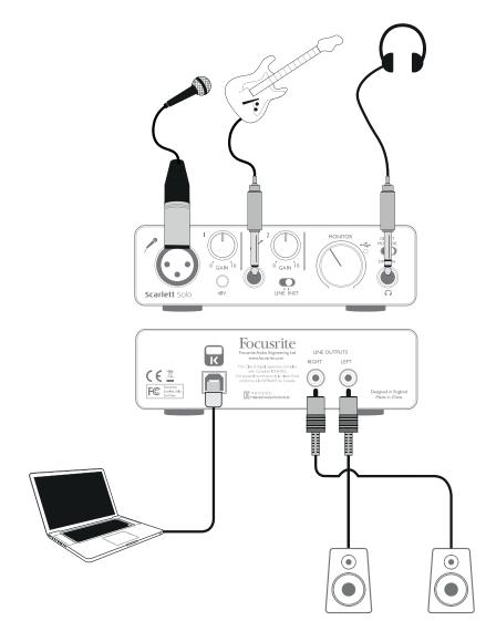
This setup illustrates a typical configuration for recording using DAW software on your Mac or PC. In this case, you might record vocals through Input 1 and guitar through Input 2 into your recording application, while monitoring the playback via headphones.
