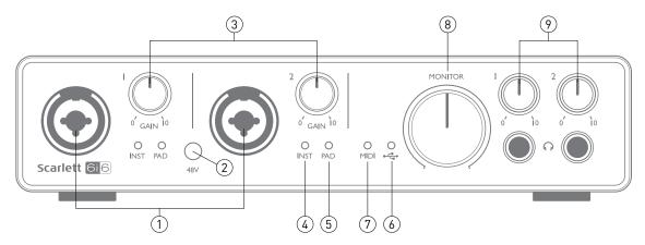
The Front Panel includes input connectors for Mic, Line and Instrument signals, the input gain and monitoring controls, and sockets for headphones.
