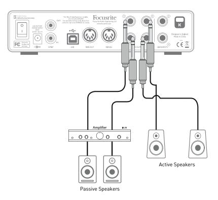
All the line output connectors are 3-pole (TRS) ¼" (6.35 mm) jack sockets, and are electronically balanced. Typical consumer (hi-fi) amplifiers and small powered monitors will probably have unbalanced inputs, either on phono (RCA) sockets, or via a 3.5 mm 3-pole jack plug intended for direct connection to a computer. In either case, use a suitable connecting cable with jack plugs at one end.
