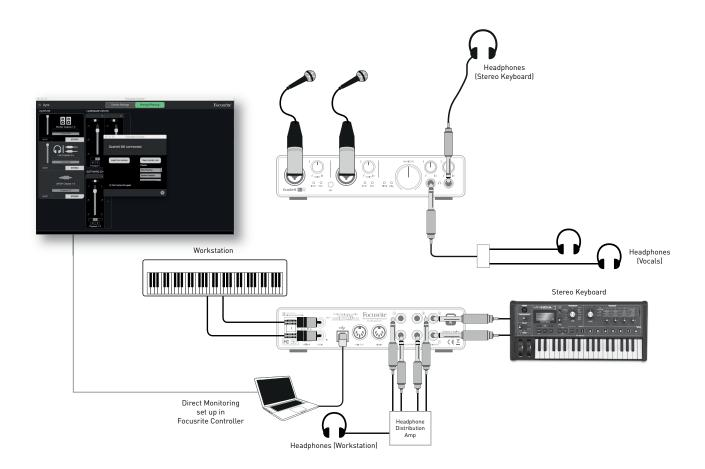
When using Direct Monitoring, ensure that your DAW software is not set to route any inputs (what you are currently recording) to any outputs. If it is, the musicians will hear themselves "twice", with one signal audibly delayed as an echo.
