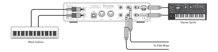
In the example illustrated, one guitar plus two stereo and one mono keyboards are connected to the six inputs of the Scarlett 6i6; Outputs 1 and 2 go to the main PA system. The player can set up a rough mix in Focusrite Control and then adjust the levels of the two mono sources against the stereo ones from the front panel.
