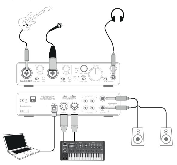
This setup illustrates the most typical configuration for recording with DAW software on your Mac or PC. In this case, you might record guitar through Input 1 and vocals through Input 2 into Ableton Live Lite, while monitoring the playback from the DAW via headphones or loudspeakers.
