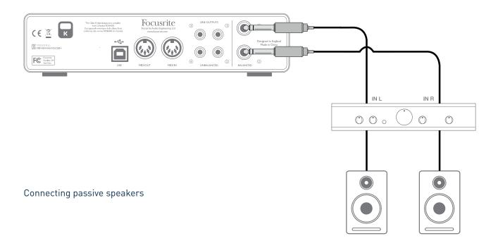
Typical consumer (hi-fi) amplifiers and small powered monitors will have unbalanced inputs, either on phono (RCA) sockets, or via a 3.5 mm 3-pole jack plug intended for direct connection to a computer. In either case, use a suitable connecting cable with phono plugs (RCA jacks) at one end. Hi-fi amplifiers and powered monitors will have their own volume controls; use these to adjust the monitoring volume.
