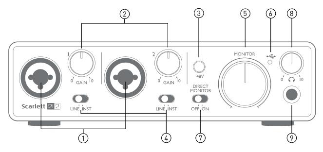
The Front Panel includes the input connectors for Mic, Line and Instrument signals, as well as the input gain and monitoring controls.
