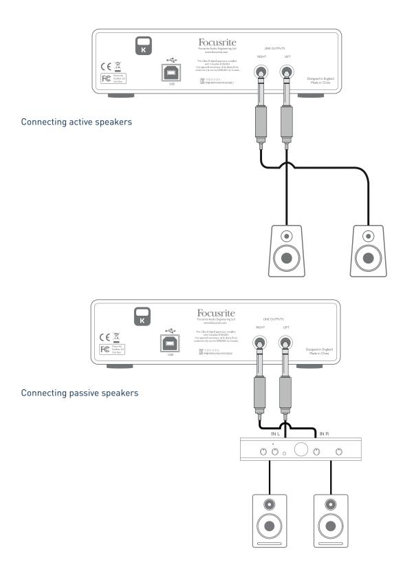
The line outputs are 3-pole (TRS)  $\frac{1}{4}$ " (6.35 mm) jack sockets, and are electronically balanced. Typical consumer (hi-fi) amplifiers and small powered monitors will have unbalanced inputs, either on phono (RCA) sockets, or via a 3.5 mm 3-pole jack plug intended for direct connection to a computer. In either case, use a suitable connecting cable with jack plugs at one end.
