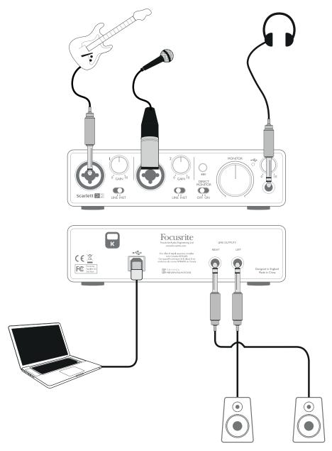
This setup illustrates the most typical configuration for recording with DAW software on your Mac or PC. In this case, you might record guitar through Input 1 and vocals through Input 2 into your DAW, while monitoring the playback from the DAW via headphones (or speakers).
