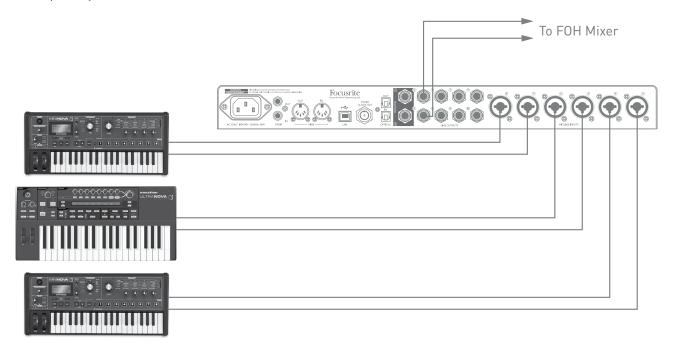
In the example illustrated, three stereo keyboards are connected to the rear panel inputs of the Scarlett 18i20; Outputs 3 and 4 go to the main PA system. The performer can adjust the volume of the individual keyboards from the front panel; he/she can also adjust the overall level of the keyboard mix.
