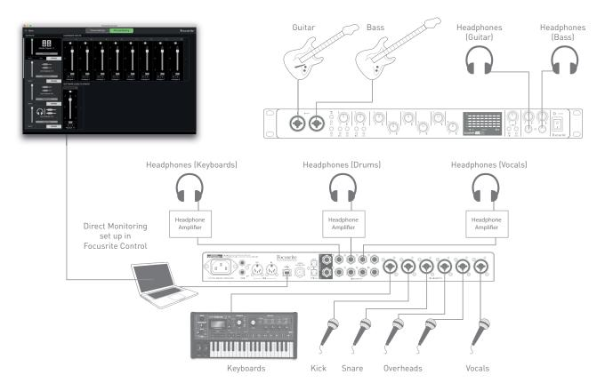
When using Direct Monitoring, ensure that your DAW software is not set to route any inputs (what you are currently recording) to any outputs. If it is, the musicians will hear themselves "twice", with one signal audibly delayed as an echo.
