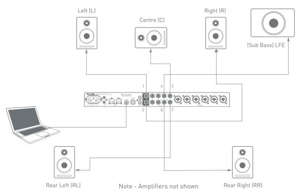
The table below summarises how some common multichannel formats could be mapped to the Scarlett 18i20's outputs for monitoring purposes, as configured within the DAW:
