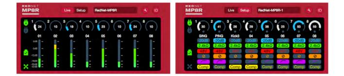
The illustration above shows the RedNet MP8R RedNet Control image. The signal level, gain and input function settings are indicated for each channel. Use the Live and Setup buttons at the top of the graphic to change view.
