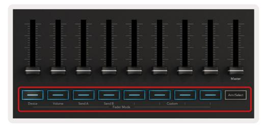
When you move a pot or fader the screen momentarily displays the parameter and its current value. You can assign these modes to either pots or faders at any given time, but both cannot have the same assignment
