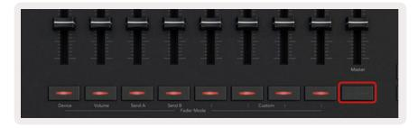
Unlit fader Buttons show no track is associated with that fader channel.
