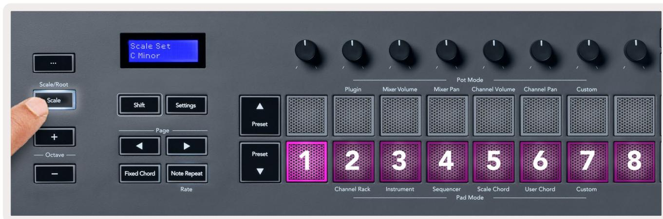
The bottom row of pads light so you can select a scale, the screen shows the selected scale. From left to right the pads select the following scales:
