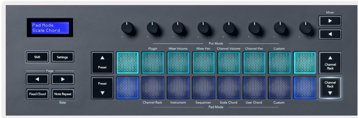
The first and last pad of each row lights up brighter than the middle pads to show root chord position. To navigate between pages of chords use the Page ◀ ▶ navigation buttons. This mode has three pages with predefined chords: Triads, 7ths, 9ths, 6/9ths
