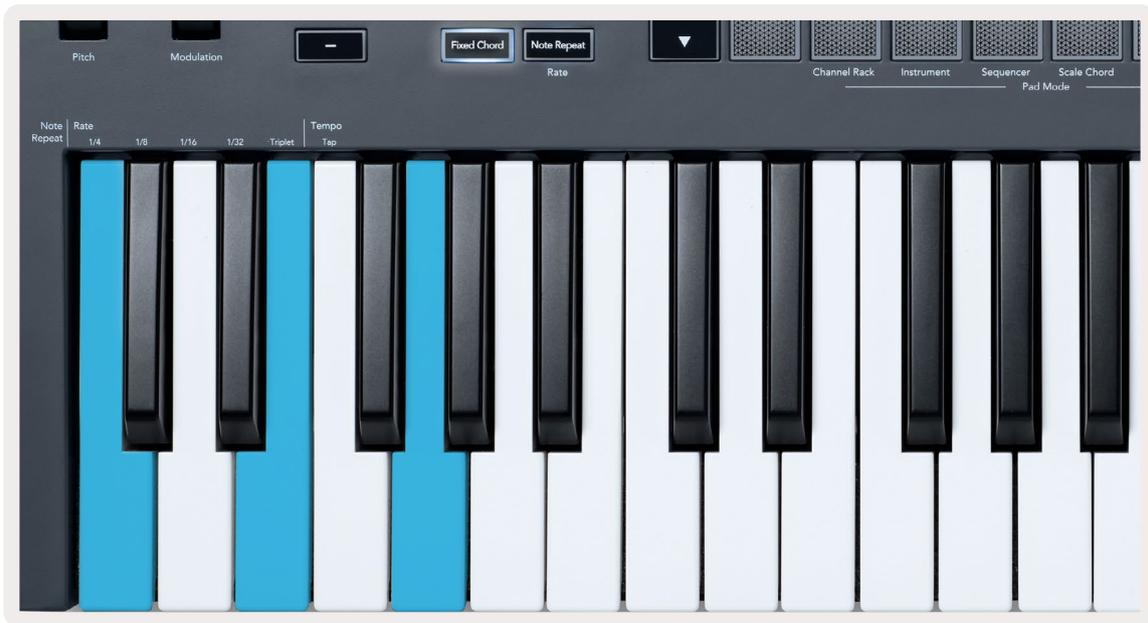
Press and hold the Fixed Chord button, press and release C, E, and finally G (a C Major chord). The FLkey stores this as the 'Fixed Chord'. Release the Fixed Chord button.
