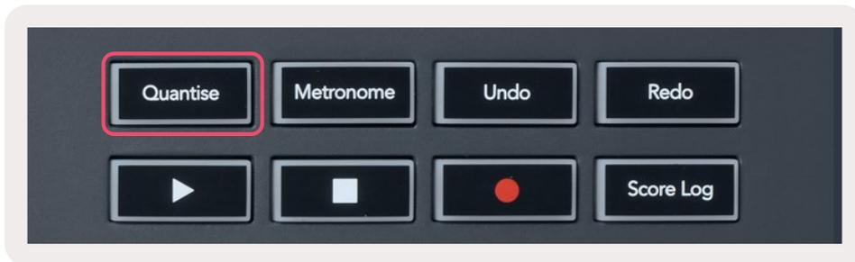
When you press the Quantise button on FLkey 37 it performs the 'quick Quantise start times' function in FL Studio. This quantises all notes start positions in the piano roll for the currently selected Channel Rack channel to the current piano roll snap setting.
