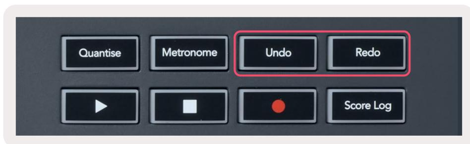
You can press the Undo and Redo buttons on FLkey to trigger FL Studio's undo and redo functions. The FL Studio setting "Alternate undo mode" doesn't affect how these buttons work.
