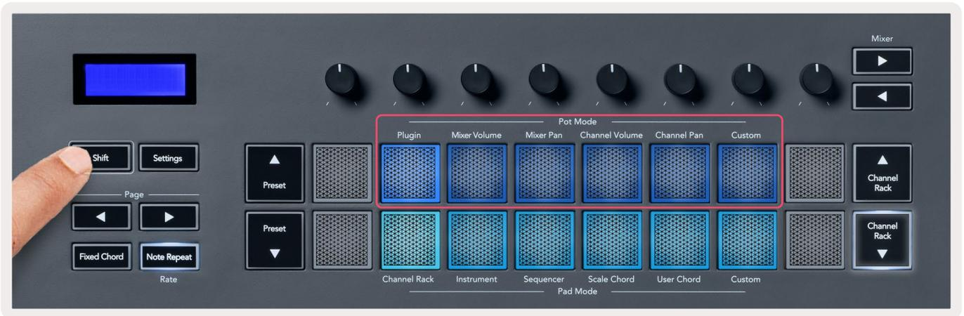
When you enable 'Pickup (takeover mode)' inside FL Studio's MIDI settings, the pot needs to reach the original value before the changes apply to the parameter connected to the current pot.
