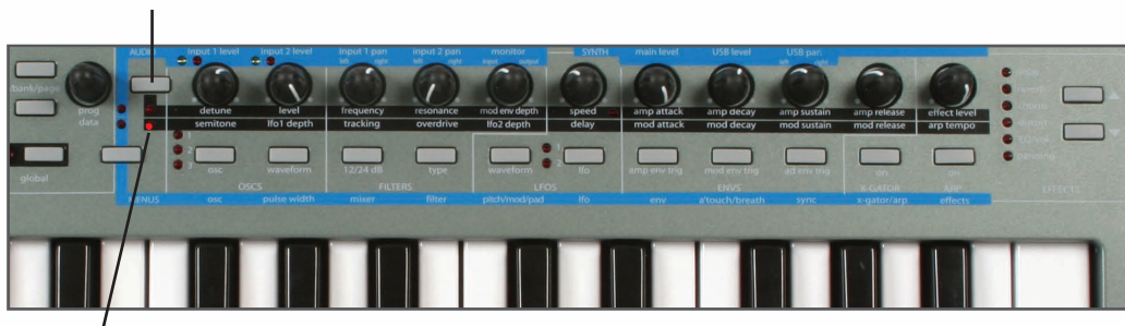
With the lower LED lit, the bottom row of parameters is active
