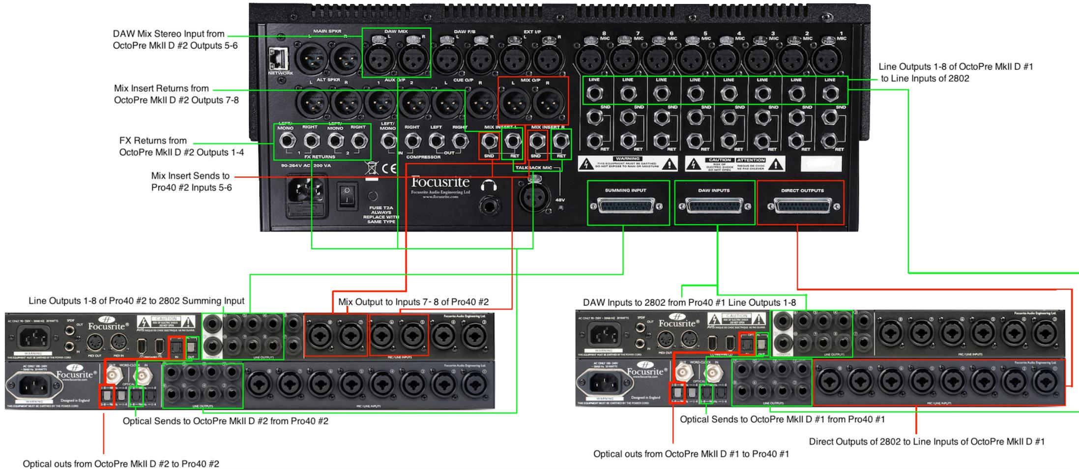
\* Please note - Pro Tools (non-HD) will only address the first 32 inputs/outputs of any system. As such, some of the features of this setup will not work exactly as shown in this diagram, some inputs/outputs may need to be shifted to account for this.
